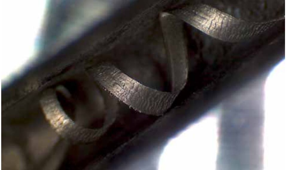
Metallic chip in spiral form.
