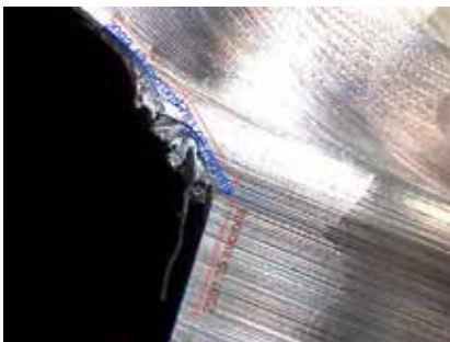
Burr remains after milling.
